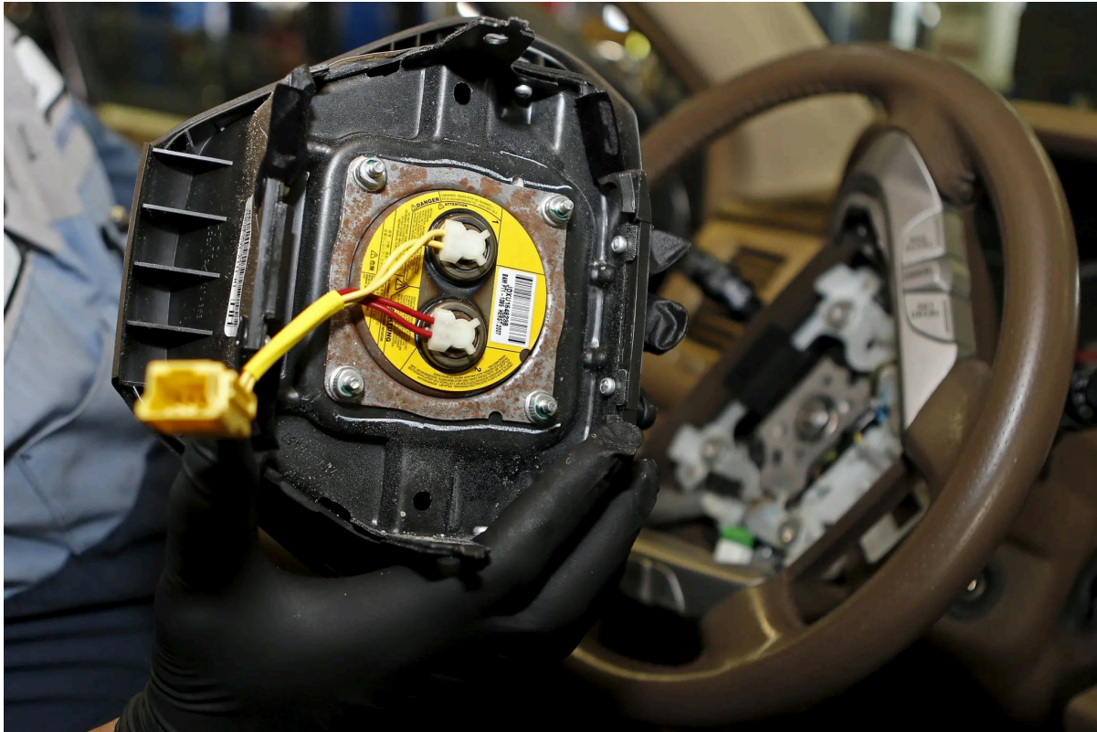
A technician holds a Takata airbag removed from a Honda Pilot in Miami. The inflator is the circular device in the center. Joe Skipper/Reuters
